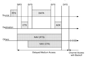
Figure 1. IEEE 802.11 four-way handshake.
