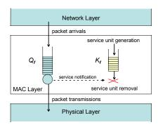
Fig. 1: A combined packet-queue  $Q_f$  and service meter  $K_f$ , for a given traffic flow f. Solid arrows represent the flow of packets/units, whereas dotted arrows represent the interaction among different system components. In the case of shared transmitters, a different pair  $(Q_i, K_i)$  is maintained at the node for each local flow i. The node transmitter notifies the service meter  $K_f$  upon completion of an f's transmission, to subtract the amount of service received.
