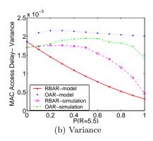
Figure 5: Expected value and variance of medium access delay for RBAR and OAR as a function of channel quality.
