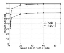
Figure 14: Throughput as a function of queue size.
