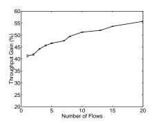
Figure 6: OAR throughput gain as a function of the number of flows.
