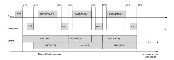
Figure 3: Illustration of fragmentation in IEEE 802.11
