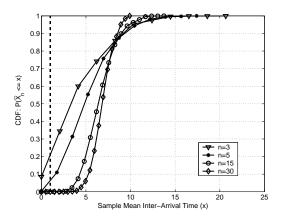
Fig. 8. Cumulative Distribution Function for request inter-arrival time:  $P(\overline{X_n} \le x)$  with varying session lengths or sample sizes 'n'.
