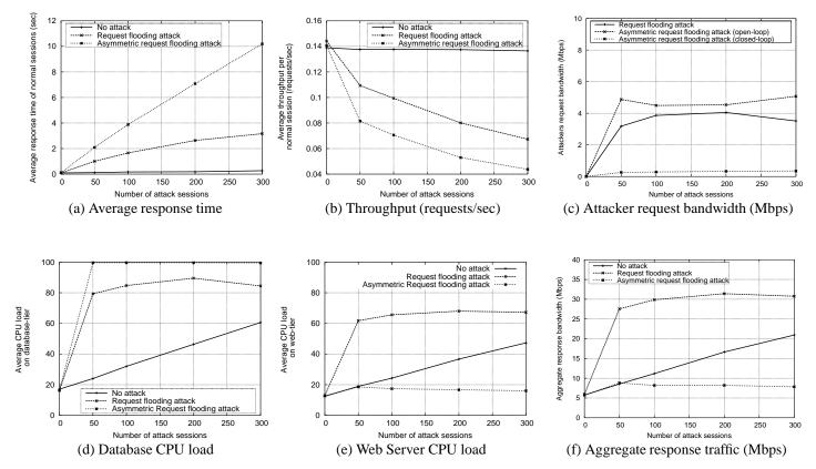
Fig. 5. Effect of most potent request flooding attack (attacker think-time=0 sec) and asymmetric request-flooding attack (attacker uses "BestSellers" script) on 100 normal sessions.
